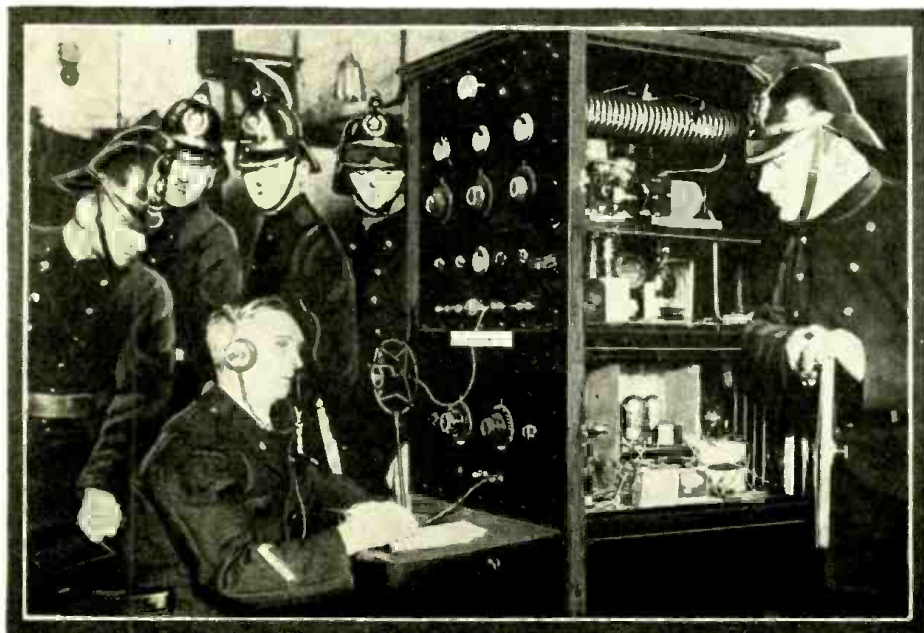
Left: English police operator at short wave transmitter receiving an important hurry call. Note "mike" for voice transmission.
