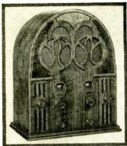
Two-dial "dual" receiver, tunes from 20 to 600 meters; without "plug-in" coils.
